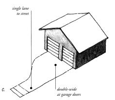
8.8a, b, c: Porous pavers provide adequate support for vehicles, yet eliminate many of the problems of conventional asphalt or concrete driveways such as heat absorption, storm water runoff, and flooding. Here are three ideas for reducing driveway pavement. Credit: Tom Richman Associates.
